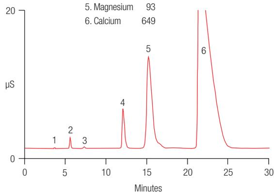
Figure 4. Determination of inorganic cations and ammonium in acidic soil extract with the Dionex IonPac CS16 column.
