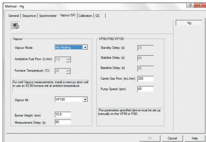
Figure 3. Settings with the SOLAAR software for vapor generation.
