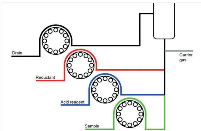
Figure 2. Schematic of the VP100 vapor generation accessory showing how the sample, acid and reductant are mixed.
