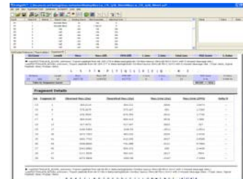
Figure 10. Using ProSightPC software, the disulfide linkage between LSFNPTQLEEQCHI and WENGECQAQK was confirmed by searching using WENGECQAQK as a chemical modification to the other chain.
