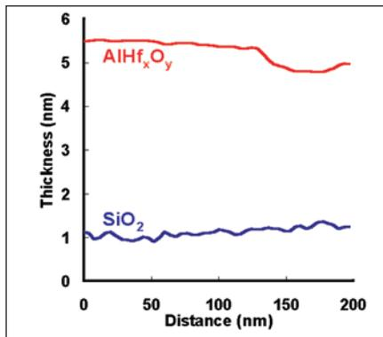
Figure 3: Thickness line scan across the diameter of the 200 mm wafer showing the variation of the thickness of the mixed Al<sub>2</sub>O<sub>3</sub> and HfO<sub>2</sub> layer and the thickness of the SiO<sub>2</sub> interfacial layer.
