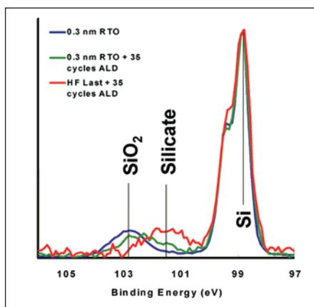
Figure 7: Comparison of Si 2p spectra from thin silicon dioxide (nominally 0.3 nm), with HfO<sub>2</sub> grown by ALD and an HF-last surface with HfO<sub>2</sub> grown by ALD.
