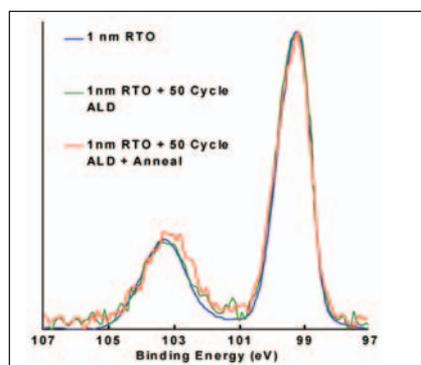
Figure 9: Comparison of Si 2p spectra from thin silicon dioxide (nominally 1.0 nm), with HfO<sub>2</sub> grown by ALD on a 1 nm RTO and following annealing at 700 °C.
