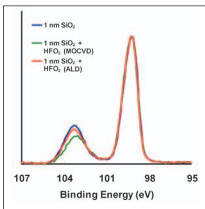
Figure 6: Comparison of Si 2p spectra from silicon dioxide (nominally 1.0 nm), with HfO<sub>2</sub> grown by ALD and MOCVD on the same material.
