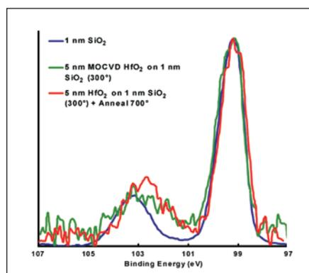
Figure 8: Comparison of Si 2p spectra from thin silicon dioxide (nominally 1.0 nm), with 4 nm HfO<sub>2</sub> grown by MOCVD on a substrate at 300 °C and following annealing at 700 °C.
