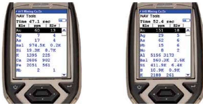
The Thermo Scientific Niton XL3t GOLDD+ XRF analyzer is used to not only identify gold grains, but also to quantify them.
