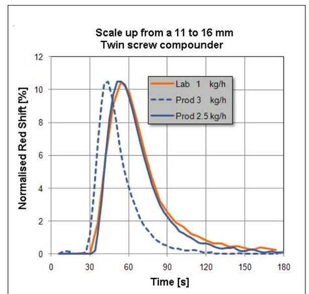
Fig. 6: Residence time for scale up tests
