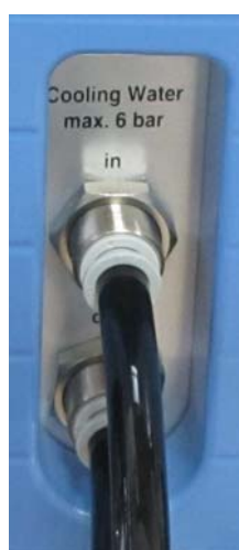
Figure 5-1. Cooling water connections at the left of the iCAP Q system
