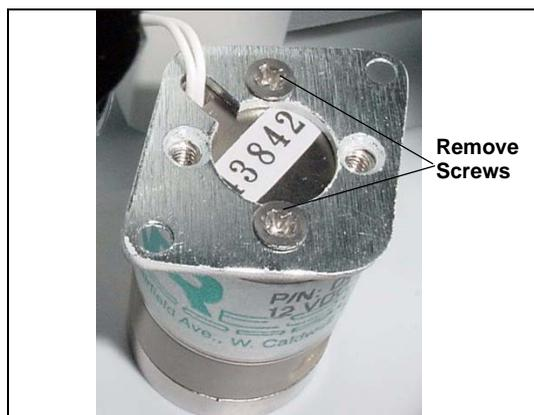
Figure 5-24. Removing the Valve Mounting Plate
