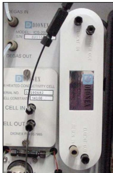
*Figure B-21. Suppressor Installed (SRS Shown)*
