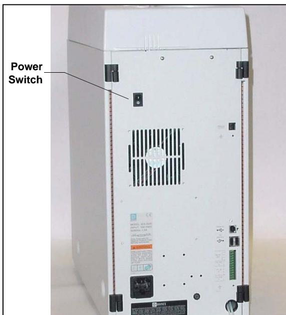
Press the power switch on the ICS-1500 rear panel (see [Figure 3-3](#)) to turn on the system power. [Table 3-1](#) shows the ICS-1500 conditions at power up.
