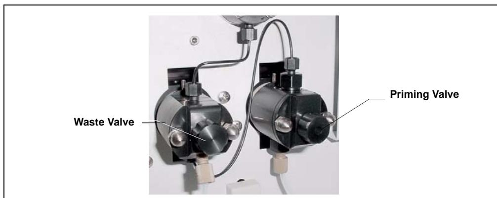
Figure 4-2. Waste and Priming Valves
