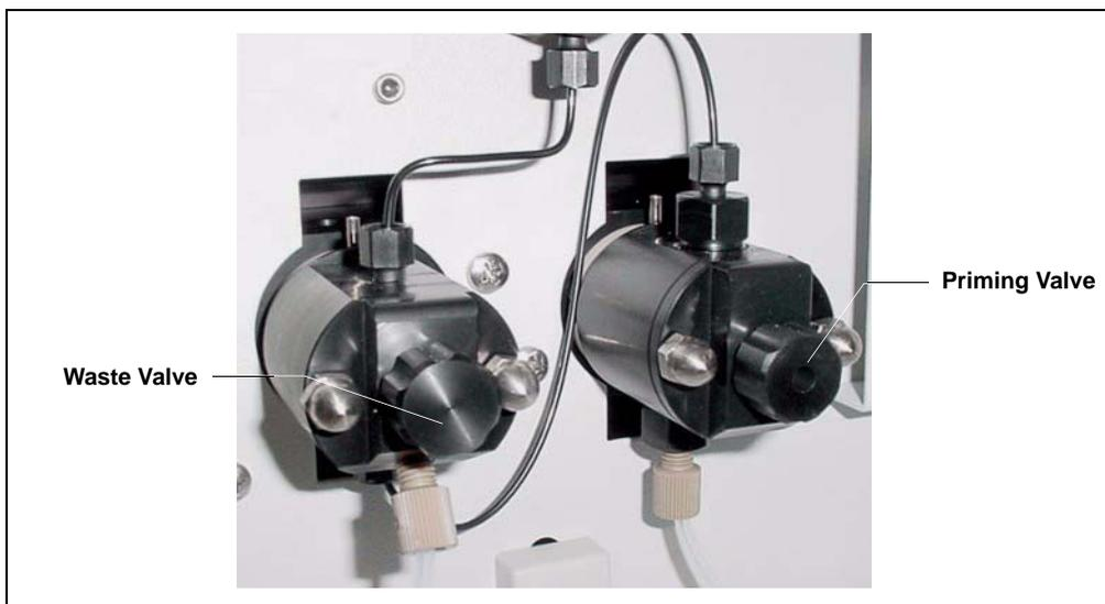
*Figure 5-12. Waste and Priming Valves*
