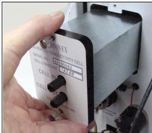
Figure 5-15. Removing the Cell Assembly
