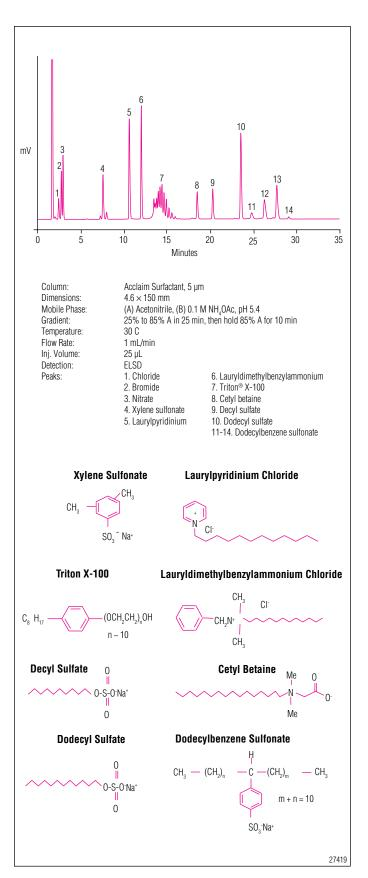
Figure 1. Simultaneous separation of inorganic anions, hydrotropes, cationic, nonionic, amphoteric, and anion surfactants.
