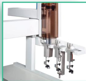
The derivatization prep cycle can handle the entire process unattended and reliably. It offers the possibility of adding derivatizing agents and internal standards, vortexing and incubating samples into an oven or into cooled trays, according to the protocol followed, for a user-selectable time. At the end of a derivatization batch, samples can be automatically injected by the same sampler into a GC or a GC/MS.
