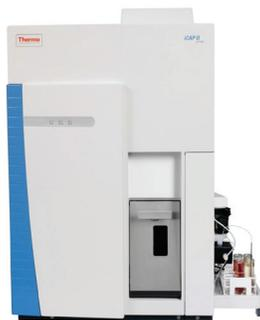
FIGURE 1. Thermo Scientific iCAP Qc ICP-MS
