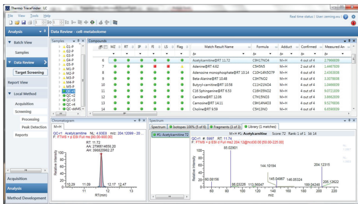
FIGURE 6. TraceFinder software squeezes all LC-MS data to automate qual/quant information extracting of the metabolome, i.e. XIC within narrow mass tolerance for relative quant and qual confirmation combining exact m/z , fine isotopic pattern, characteristic fragments, reference MS^2 spectrum as well as retention time.
