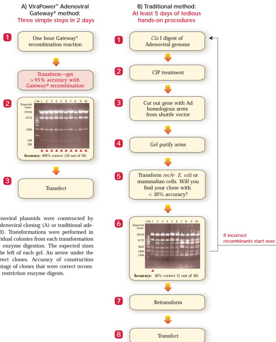
Recombinant adenoviral plasmids were constructed by either Gateway® adenoviral cloning (A) or traditional adenoviral cloning (B). Transformations were performed in parallel. Ten individual colonies from each transformation were screened by enzyme digestion. The expected sizes are indicated to the left of each gel. An arrow under the gel indicates correct clones. Accuracy of construction reflects the percentage of clones that were correct recombinants, based on restriction enzyme digests.
