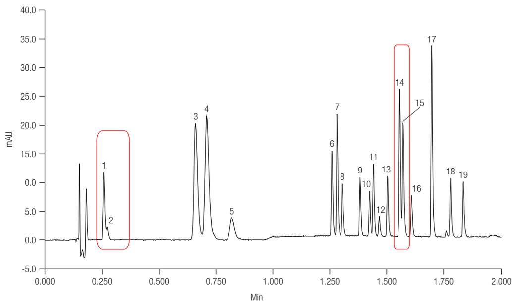
Figure 2. Chromatogram showing the separation of 19 beta blockers at a flow rate of 1.7 mL/min (back pressure 1365 bar), within a 2 minute detection window.
