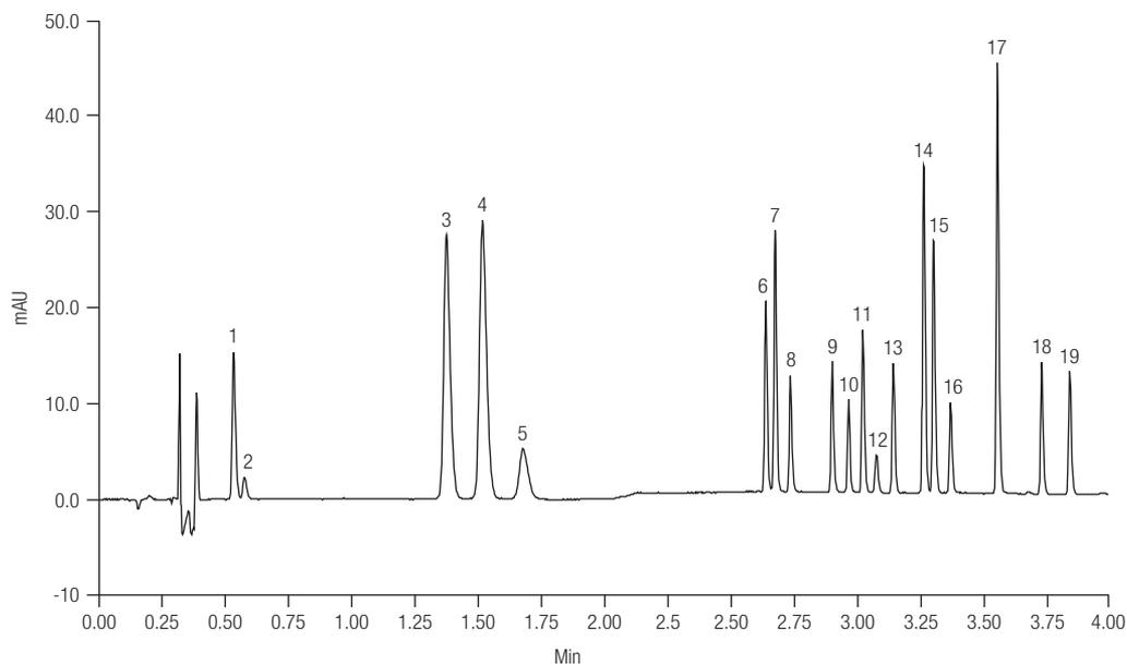
Figure 1. Chromatogram showing the separation of 19 beta blockers at a flow rate of 0.8 mL/min (710 bar back pressure), within a 4-minute detection window.
