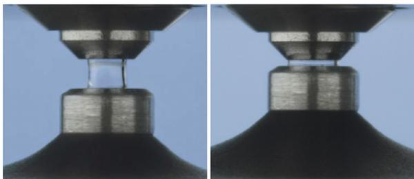
Figure 1: Sample liquid column during measurement, showing the 1.0 mm (left) and 0.1 mm (right) pathlengths.
