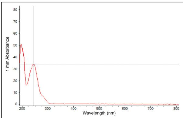
Figure 2: Absorbance spectrum of 6 mg/mL acetaminophen standard. Absorbance maximum at 244 nm was used for subsequent analysis.
