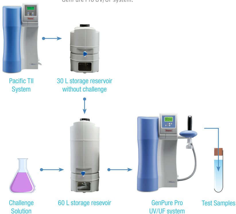
Figure 1. Diagram of a Pacific TII system with a 30 L reservoir without challenge, 60 L reservoir for challenge solutions and GenPure Pro UV/UF system.
