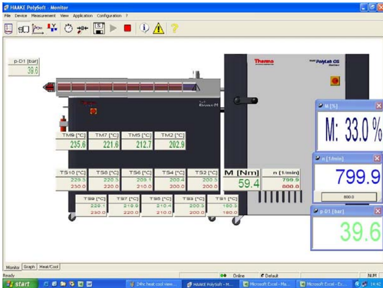
PP-Dellite compound, 30 kg/h at 75% of maximum torque.
