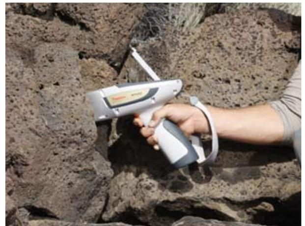
The Thermo Scientific Niton XL3 GOLDD is an ideal instrument for fast mine or field analysis.
