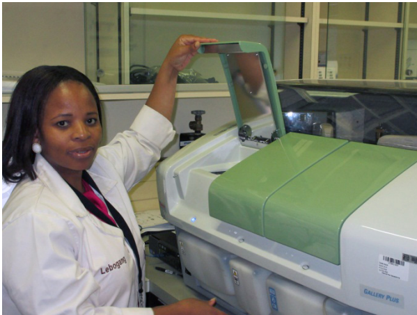
▲ Lebogang Sathekge opening the Gallery Plus analyzer sample compartment.
