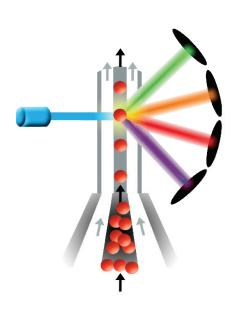
The Thermo Scientific Cyto-Cal Multifluor Calibrator contains polymer particles with dyes that excite and emit at the spectral ranges commonly used in flow cytometry..
