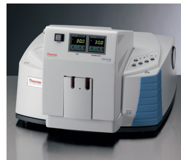
Figure 1: The Thermo Scientific Nicolet iS™ 10 FT-IR spectrometer with the TGA accessory inserted
