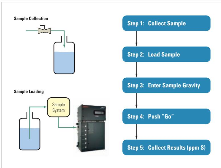
figure 3 – At-line sulfur analysis with the SOLA II
