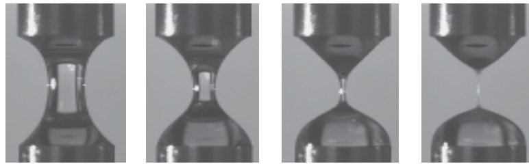
Figure 2: Sequence of a CaBER measurement [1].
