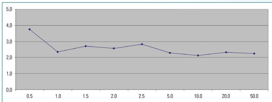
Dispensing precision (CV%) with 0.5–50  $\mu\text{l}$ . Different volumes of 0.04 M fluorescein was dispensed into black Thermo Scientific 384-well Microtiter Microplates and measured at Ex485/Em518 nm.
