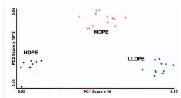
Figure 4: Principal component scores plot demonstrating clear spectral separation between the different density classes of polyethylene.
