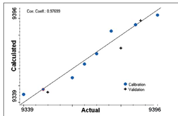
Figure 5: Regression plot showing the fit of the chemometric model for the MDPE samples. Root Mean Square Error of Prediction (RMSEP) = 0.0005.
