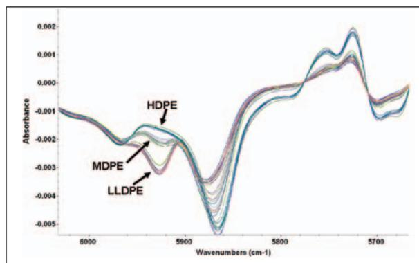
Figure 3: First derivative spectral range analyzed for discriminant analysis of the different polyethylene density classes.
