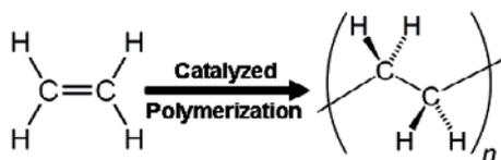
Figure 1: Catalyzed polymerization of ethene to form polyethylene
