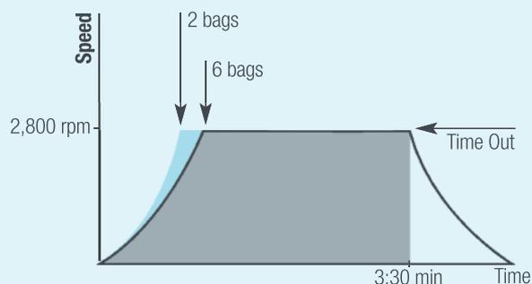
**Figure 1:** In a typical first centrifugation step, a two-bag rotor load attains set speed faster than a six-bag load. Since both loads will time out at the set time of 3:30 minutes, different g-forces are achieved during the run. By using the ACE integrator function, the time for 2 bags would be changed to 3:00 minutes to obtain the same overall g-force for both loads.
