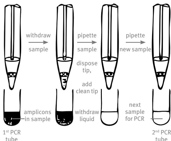
Figure 1: Use of ART Self-Sealing Barrier Tips illustrates that aerosols generated during initial pipetting steps are restricted to lower portion of the tip.
