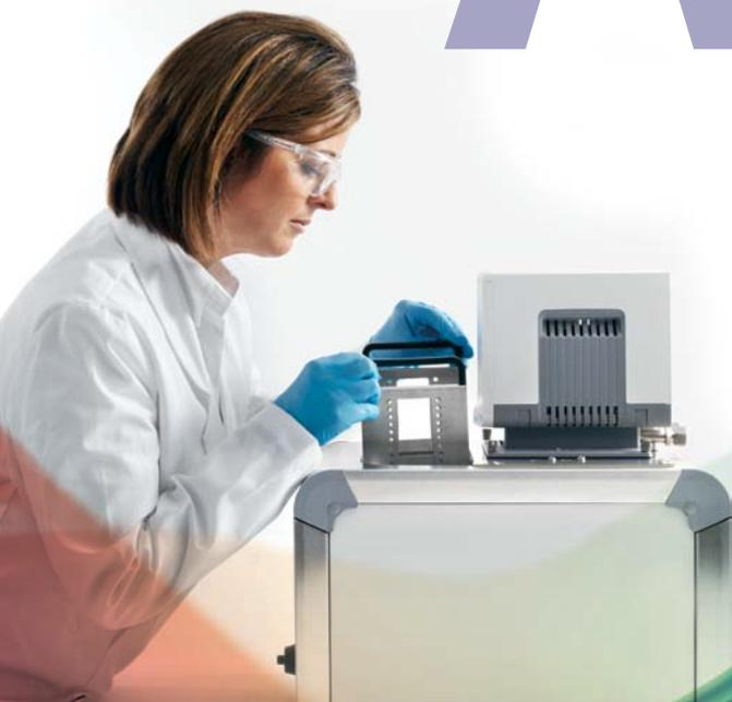
For applications requiring test tubes, Thermo Scientific™ racks are available in a variety of configurations to accommodate test tube diameters. Once the correct size test tube rack is selected, a corresponding bath that meets the temperature range and fits that rack can be selected.
