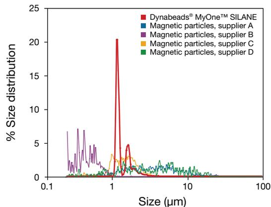
**Figure 2—Dynabeads® are monosized.** The graph shows size frequency distribution of Dynabeads® MyOne™ SILANE (red) and magnetic particles from four alternative suppliers, as analyzed by flow particle image analysis on a Sysmex FPIA-3000 (Malvern Instruments Ltd.). The second peak for Dynabeads® at 2 µm represents doublets. Monosized Dynabeads® ensure optimal, predictable behavior in automated systems. Minimal variation within and between lots allows for standardized and reproducible processes.
