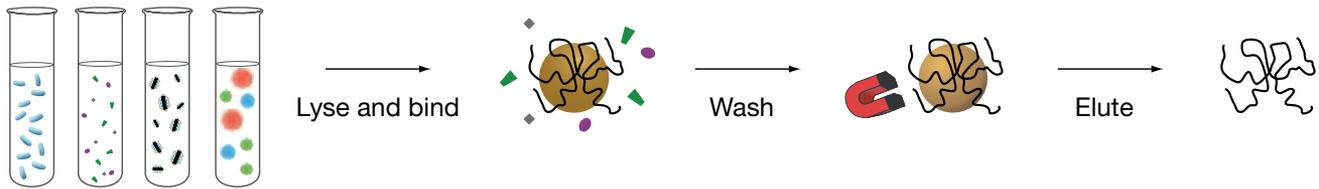
**Figure 4—Quick and automatable magnetic separation protocol.** The illustration shows the simple steps (lyse, bind, wash, and elute) of the automatable protocol for nucleic acid capture from a variety of biological samples using Dynabeads® MyOne™ SILANE.
