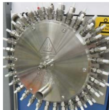
Figure 4. Rapid Multistream Sampler (RMS) with remote analyzer connection.
