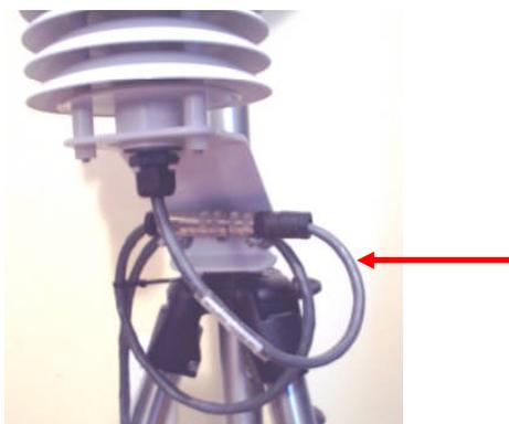
2. If you are experiencing issue with intermittent signal loss or a failed temperature reading you should open the connection at the inlet area and check for corrosion on the contacts. If corrosion is present you should replace the cables.
