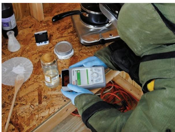
**The FirstDefender RM unit can analyze through sealed containers without disturbing the sample.**
