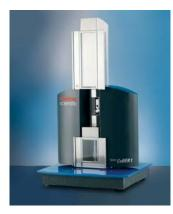
The Thermo Scientific<sup>™</sup> HAAKE<sup>™</sup> CaBER 1 instrument is the only commercially available extensional rheometer for low and medium viscous fluids. Extensional flow fields occur in many food processing steps such as filling, spraying or coating. Extensional properties
