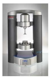
Thermo Scientific<sup>™</sup> HAAKE<sup>™</sup> MARS<sup>™</sup> instruments are highend rotational rheometers for extended material characterization, including the analysis of viscous or viscoelastic properties in rotation or oscillation modes. In addition, MARS rheometers offer normal force capabilities that enable squeeze, penetration and tack measurements of liquid or solid food products. Many accessories are available for analyzing foods:
