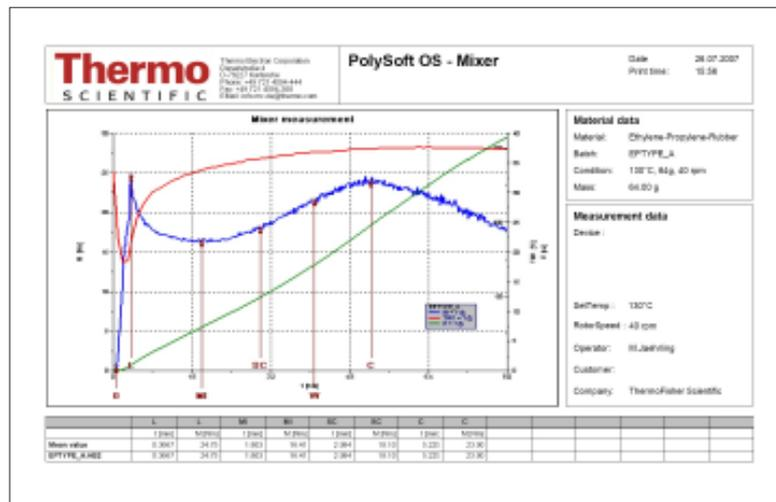
Fig. 4. Flow-curing behaviour of an EP-compound
