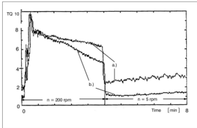
Fig. 2: Mastication test of a NR with and without "Renazit"
