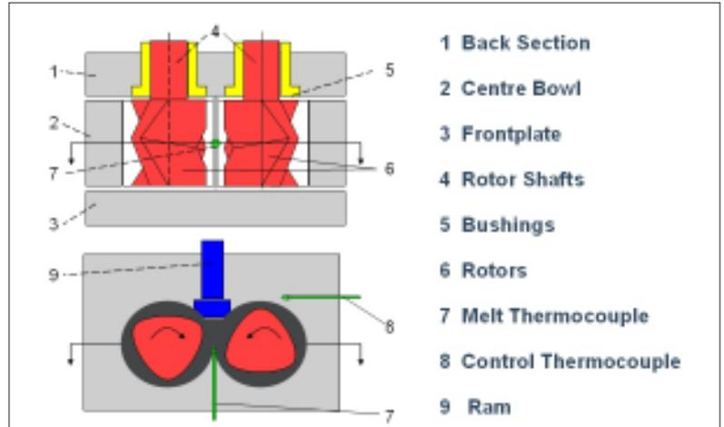
Fig.1: Principle sketch of an internal mixer
