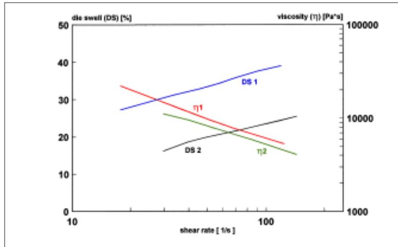
Fig. 7: Die-swell and viscosity of two rubber compounds as a function of shear rate
