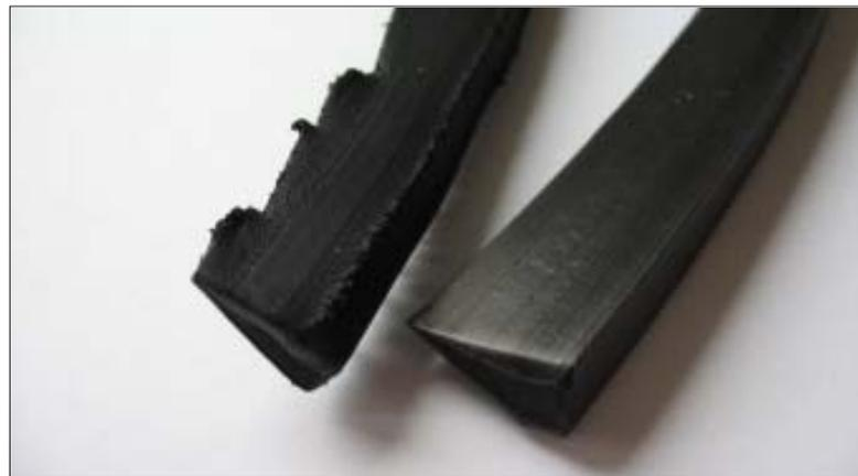
Fig. 9: Test result from a Garvey test with two rubber compounds
