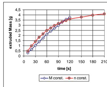
Figure 3: Comparison of extruded mass at constant speed n and at constant torque M (co-rotator).
