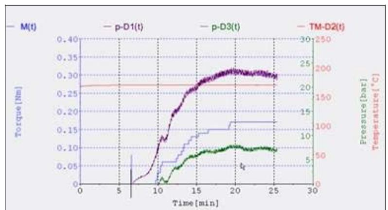
Figure 5: Monitoring the reaction time online, polymerization of L-lactid to biodegradable polymers
