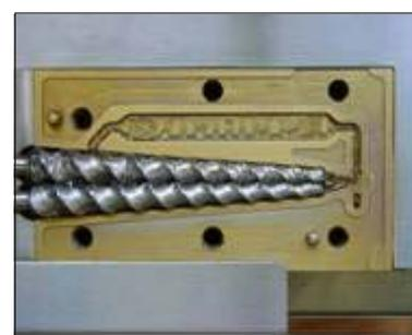
Figure 2: Co-rotating screws
