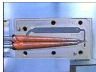
b) Asaclean (PS cleaning compound) + Remafin orange duration of the test  $t=90$  s, test condition like in Figure 4
