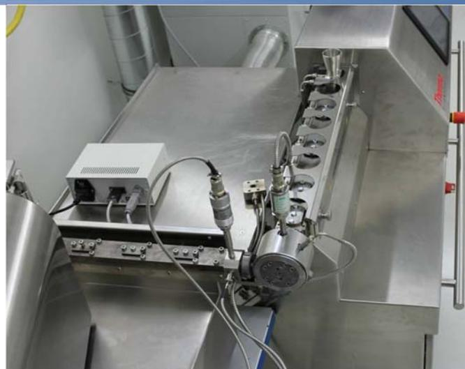
Fig. 1: Set-up of twin-screw extruders for co-extrusion.
