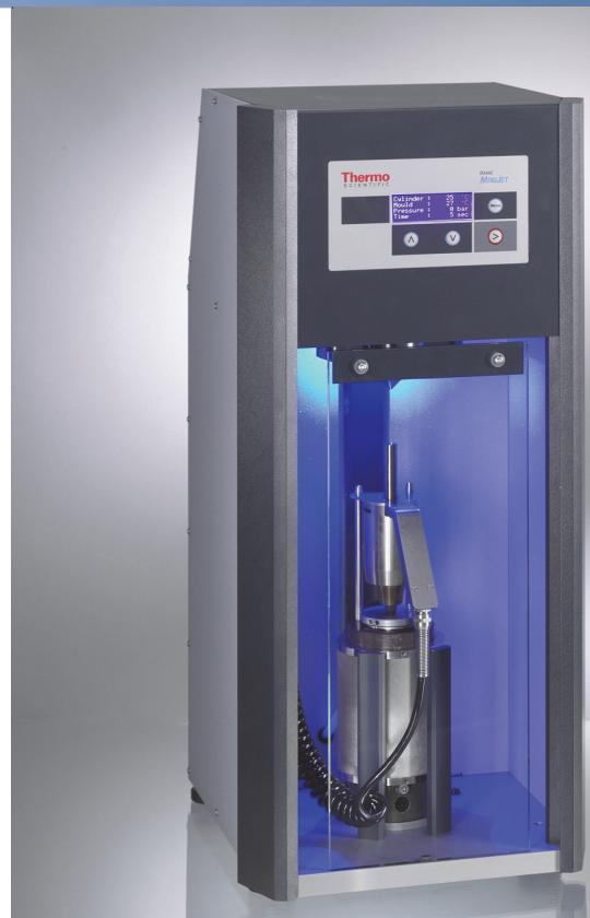
Fig. 1: The HAAKE MiniJet Pro injection molding system.
