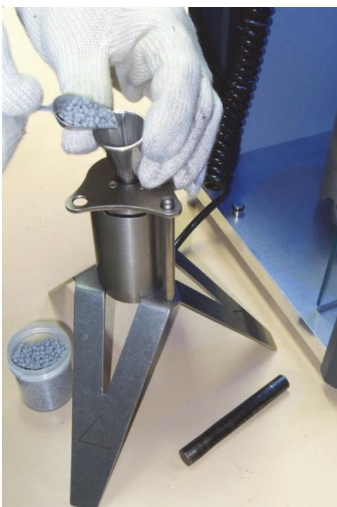
Fig. 2: Filling of pellets in the heated cylinder.
