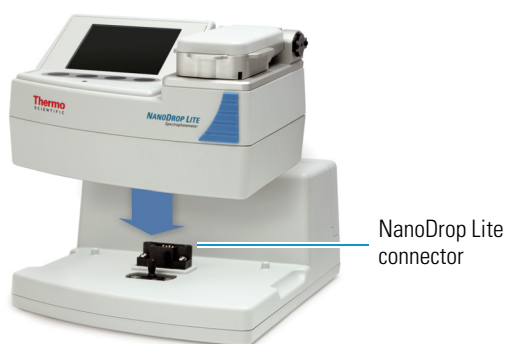
Figure 1. Connecting the NanoDrop Lite to the printer
