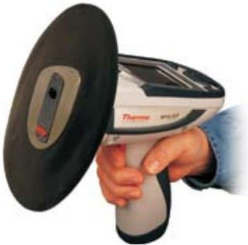
**Backscatter Shield** – This patented device prevents scattered radiation from light-matrix samples returning to your hand, especially those samples associated with consumer goods, RoHS, WEEE, and ELV analysis.
