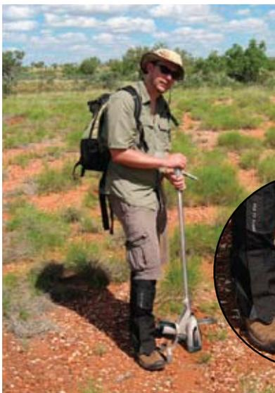
**Thermo Scientific Extend-A-Pole** – Providing dual, remote trigger activation for ease of use in multiple orientations, the telescoping extension pole features an instrument cradle that clamps to the analyzer, an adapter to hold a GPS or PDA, as well as a fixed tripod adapter.
