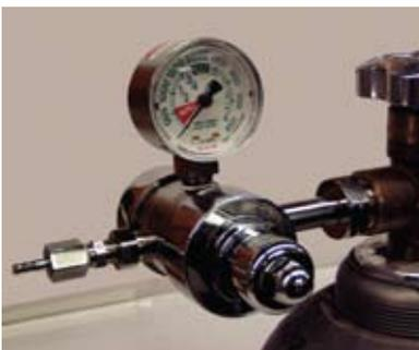
**Stationary Tank, Two-Stage Regulator** – This custom two-stage regulator for large, fixed-site helium tanks governs and optimizes gas flow at a fixed rate for Niton XL3t 900 Series Helium Purge analyzers.
