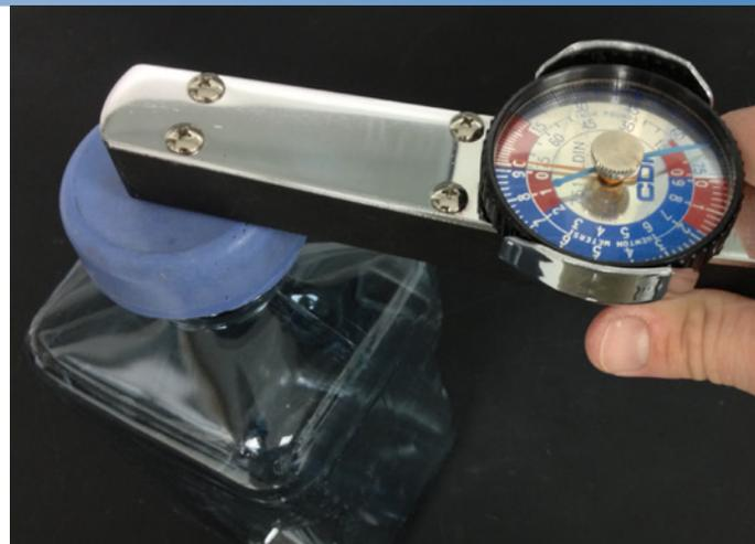
expansion and contraction of the materials at the threads and mating surfaces. This movement, in addition to the change in malleability of the resin at cold temperatures, exacerbates the back-off torque degradation.
