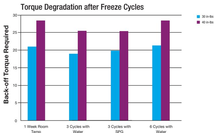
Figure 3. Back-off torque of Biotainer bottles containing water after 3 or 6 freeze/thaw cycles, Biotainer bottles containing SPG after 3 freeze/thaw cycles, or Biotainer bottles left at room temperature for a week with no freezing. All results represent data for 1L Biotainer bottles for comparison.
