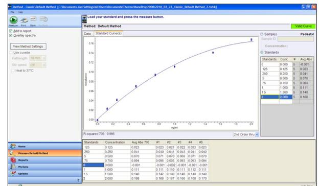
Figure 3: Standard curve for a typical Lowry assay showing the standard curve of absorbance of each standard after incubation with the Lowry reagent. Note that the relationship between the absorbance and the protein concentration is not linear.
