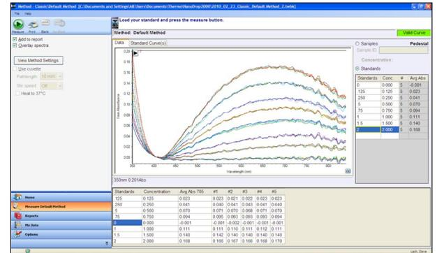
Figure 2: Standard curve data for a typical Lowry assay showing the absorbance values and spectra for each replicate.
