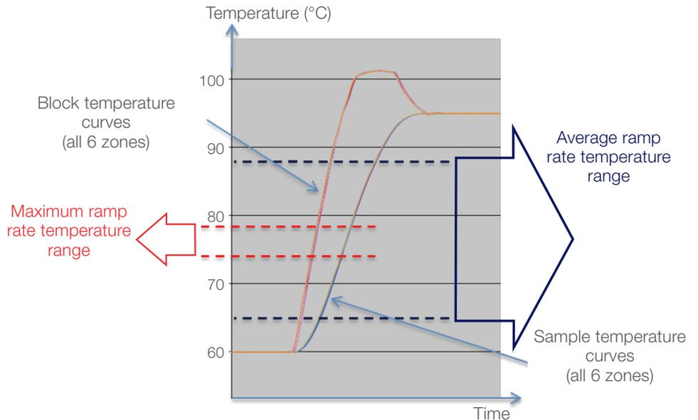
**Figure 1. Real block and sample temperature curves from all six zones during up ramp on the Applied Biosystems™ ProFlex™ 96-well PCR system.** The dotted lines indicate the temperature range sampled for the maximum ramp rate and the average ramp rate.
