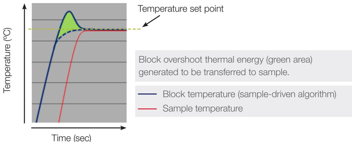
**Figure 2. Block overshoot thermal energy.** The reaction block (blue) and sample (red) temperature curves and associated block overshoot thermal energy (green) during a heating phase that is ideally controlled. The horizontal dotted line indicates the set temperature for this phase.
