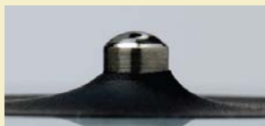
Droplet "flattens out" on unconditioned pedestal
