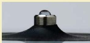
Droplet "beads up" on properly conditioned pedestal
