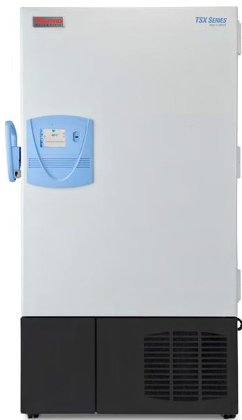
V-drive technology enables a TSX freezer's compressor to run at variable speeds depending upon the situation, while conventional compressors are forced to continually cycle on and off. The V-drive will automatically tune the BTU reserve capacity to the heat loads presented to the freezer, meaning the compressor is not forced to quickly operate at full power when the door is opened.
