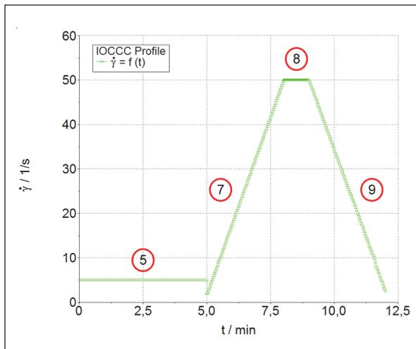
Fig. 2: Shear rate profile applied according to ICA method 46. The numbers 5 to 9 represent the job element number of the HAAKE RheoWin job shown in Figure 3.
