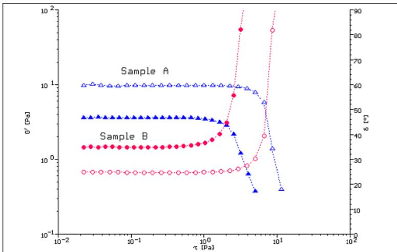
Figure 4: Amplitude sweeps at 1 Hz for two suspensions
