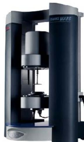
Figure 1: HAAKE MARS a Modular Advanced Rheometer System
