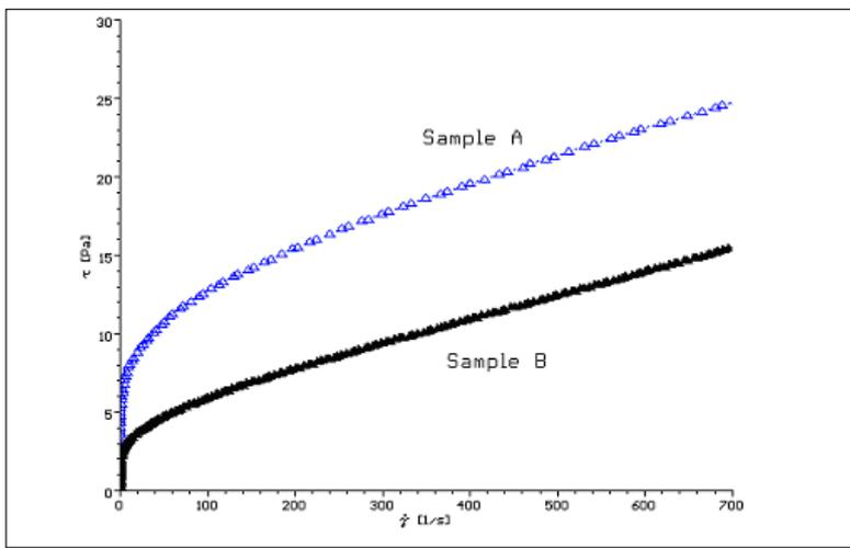
Figure 2: Flow curves of two suspensions
