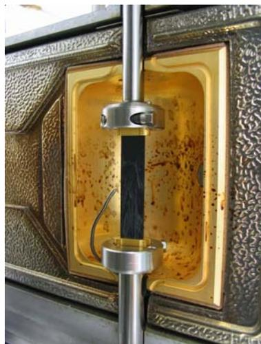
Fig. 1: Solids clamps holding a solid sample in front of the right half of the CTC
