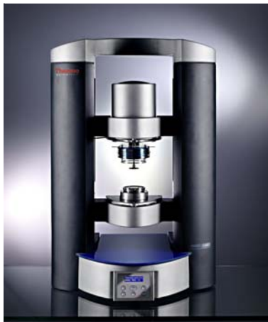
Fig. 2: Thermo Scientific HAAKE MARS rheometer platform for individual configuration
