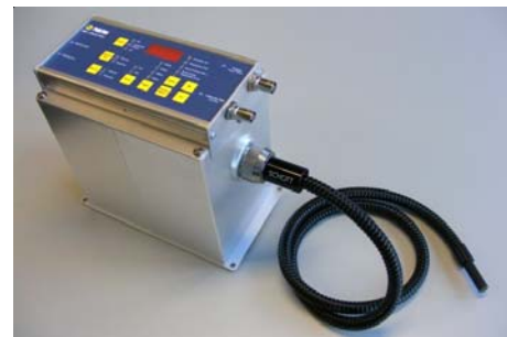
Fig. 3: Stroboscope (BVS-II Wotan, Polytec GmbH), equipped with a Xenon flash lamp, maximum flash frequency 20 Hz (200 Hz with internal trigger).
