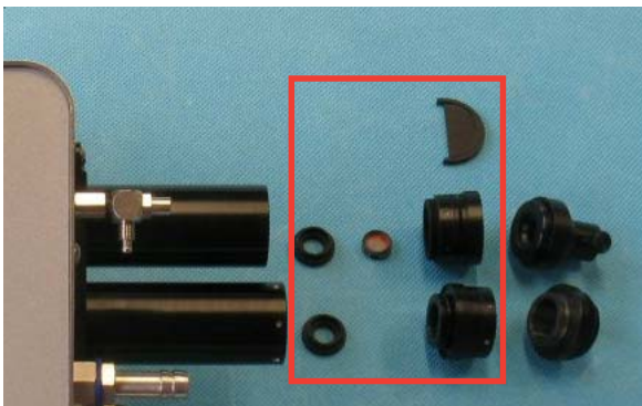
Fig. 7: Optional segment universal holder (red box) for HAAKE RheoScope lighting tube (center left) and/or camera tube (bottom left), offering a slit to mount a half circle diaphragm (top) as well as a mounting ring for a standard filter with a 12.5 mm metric thread (center).
