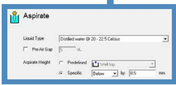
**Caution:** When using a "Specific Height" in a sequence, ensure the vessel type selected in the "Move To Position" that proceeds the "Aspirate / Dispense" step uses this same specific liquid handling depth as appropriate. Verify the same specific height is entered for any other steps that use it in the sequence for consistency.
